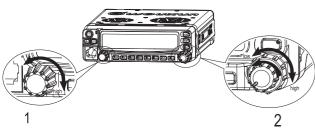
Turn the volume knob clockwise to increase the volume and the RX volume. The maximum volume is level 16. Turn the knob counter-clockwise to decrease the volume and the RX volume. Continue turning the knob counter-clockwise to shut off.
